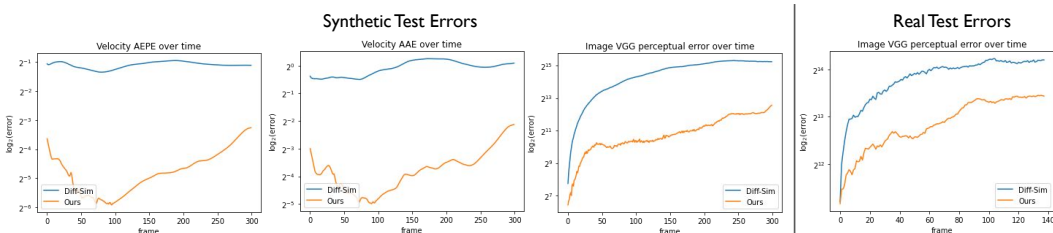
Figure 11: Error plots of the comparison between Diff-Sim and our DVP method on a synthetic dataset.
